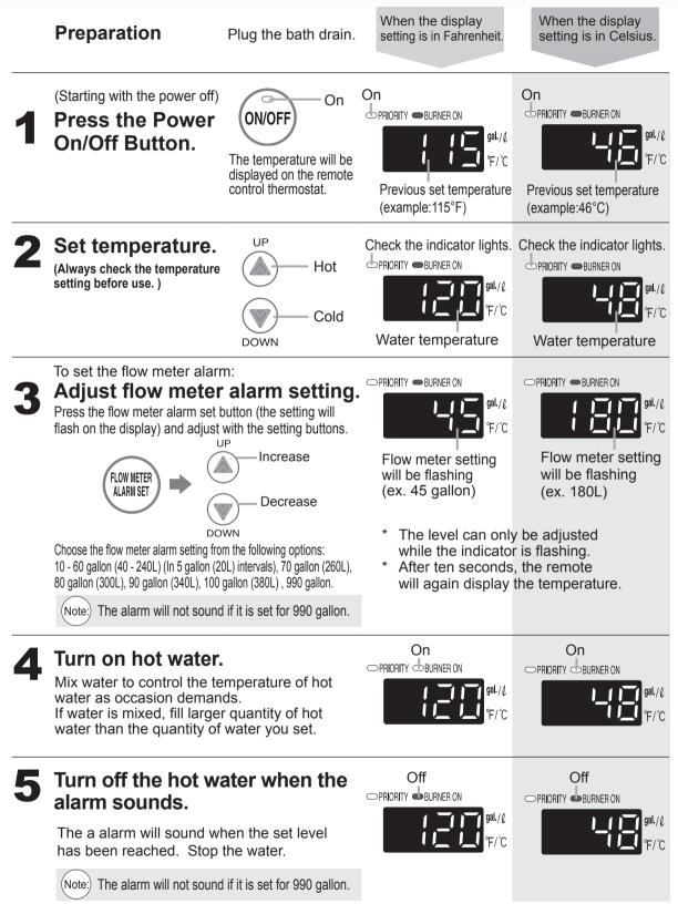
An alarm will sound for ten seconds when the flow reaches the set level.
